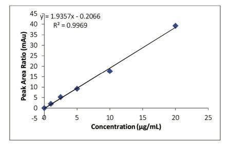
Figure 2. HPLC calibration curve for DL-alpha tocopherol
